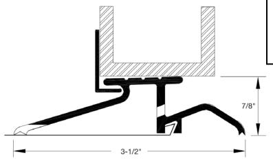
T150 pan and factory drilled weep holes are available.  $\#10 \times 1-1/2$ " wood screws provided.
